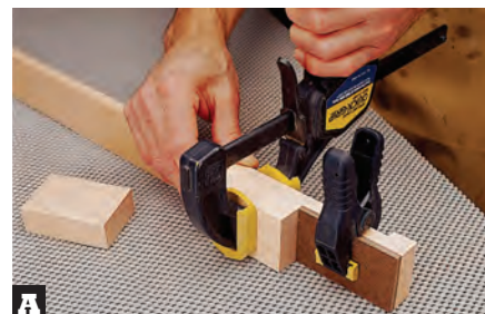
A Clamping the spacer jig to the rails helps you accurately position the end spacers.
