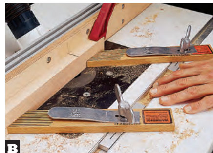
B Mark the bit location on your fence. Stop routing when the stop line on the extension aligns with the mark on the fence.
