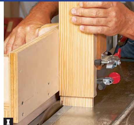
I On wider stock, Zane nixes the spacer and relies on the outer clamp to secure the workpiece when cutting cheeks.
