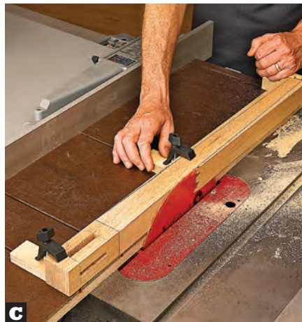
C Hold the taper jig tightly against the table saw rip fence as you cut. Before starting each pass, make certain that your left hand is well away from the line.
