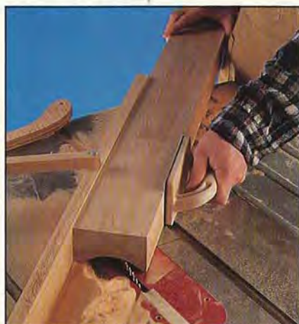
Masking tape, foreground, covers the unused opening in the tablesaw insert to reduce the flying sawdust.
