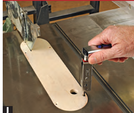
J Adjust the leveling hex screws to ensure the insert sits flush with the tablesaw's top. If it sits too high your workpieces will catch on it.
