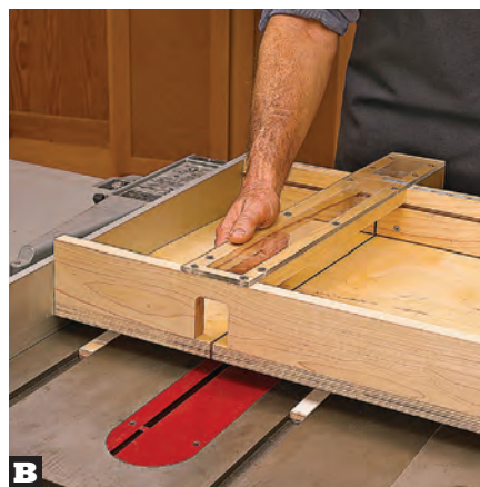
B Keeping the right end of the platform against the rip fence, set the sled assembly on the guides. Press down firmly to stick the bars to the platform.
