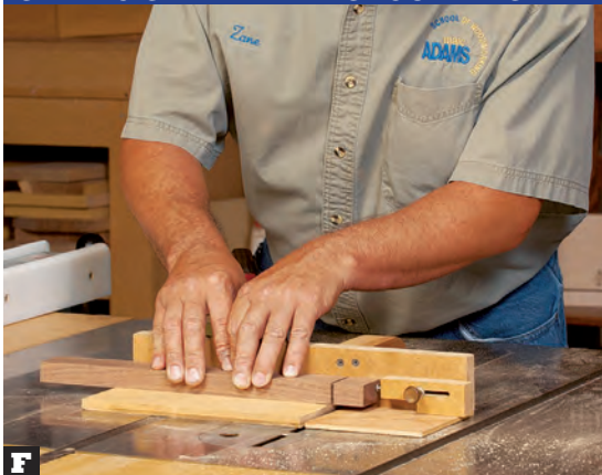
F Raise the blade to the establish the needed tenon depth. Then, using the jig, cut shoulders on the workpiece faces and edges.
