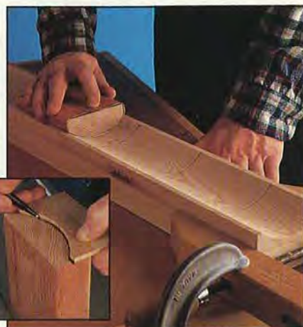
As you sand the cove molding, be careful to remove only the saw marks. Smooth with 100- and 150-grit papers.
