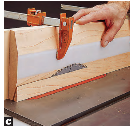
C A carrier board stabilizes the glide top for bevel-ripping.
