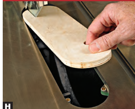
H Place thumbtacks onto the ledges, and then gently lower the insert into place. Tap it lightly to make indentations.
