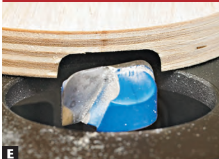
E Use any bit that can rout a channel. We used this dish-carving bit to create a 3/4"-wide relief necessary for a 45° bevel cut insert.
