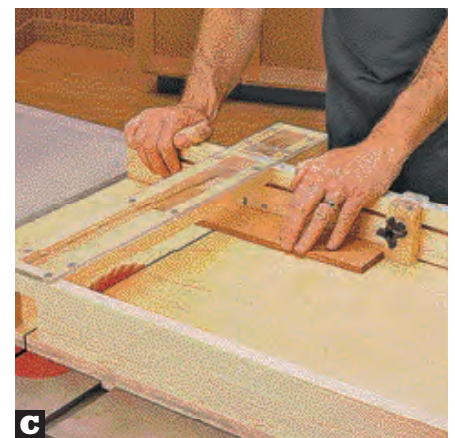
C Hold the workpiece firmly against the fence as you make a cut. Keep your hands outside the blade guard, and don't cut through its end.
