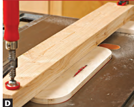
D Because the insert rests on top of the saw, secure it firmly with double-faced tape and a board and clamps.
