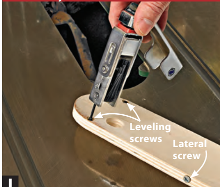
I Add hex screws for leveling. Add wood screws to one edge and end for lateral adjustments if the insert is too loose.
