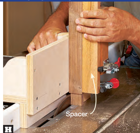
H When cutting edge cheeks, Zane sometimes places a spacer between the opposite edge and outer clamp to achieve a firm hold.
