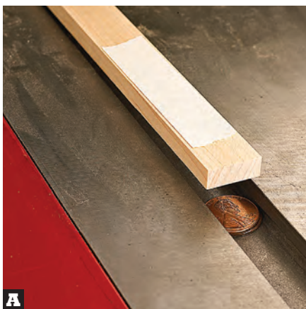
A Two pennies shim the miter-slot guide bars slightly above the tablesaw surface. Place a couple of these stacks in each miter-gauge slot, and set the bars on top.
