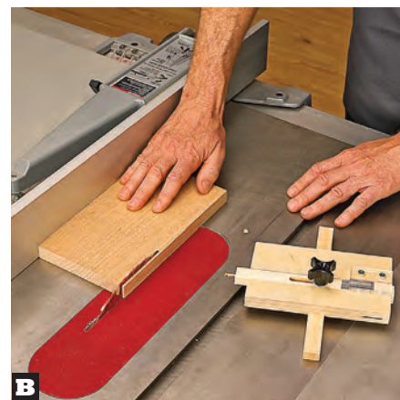
B To cut spline stock, use the thin-strip ripping jig (see the how-to details, beginning on page 5) to cut spline stock. Reposition the fence between cuts.
