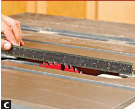
C With this steel rule resting on the insert ledges, you can see that the 10" blade requires a relief cut in a blank insert.
